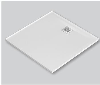
**STEP 1** Measure outside edge of Profile base . Oceano's manufacturing process has a tolerance of + or - 2mm, so it is important to measure the outside edge of the Profile base so the correct thickness mortar bed can be levelled within the rebated area of the bathroom.
