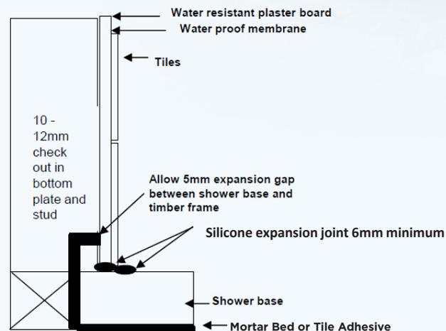
**STEP 8** Once base is installed and cured run a silicone bead around outside edge of the base and floor to create an expansion seal.
